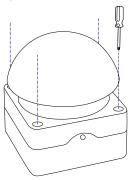
Unscrew the top part of the button from the base, to get access to the battery. Replace the battery with a Lithium Metal 3V CR123 size battery (also called 123A or A123 size).
