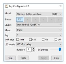
The utility configures only a single button at a time. The serial number, at the top right, shows which button is being configured.
