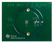
The rationale is that the board has an RF-connector, for easy connection to a VNA (vector network analyser), a short trace designed to have an impedance of  $50\Omega$ , and a set of footprints on that trace for mounting the various configurations of (parallel) capacitors.
